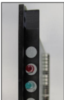
Figura 125: TMEW2 – LED de la placa frontal
